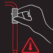
**⚠ For best performance and hygienic purposes, a steam out of 5 seconds minimum MUST be done before and after each usage to avoid milk residues from remaining inside and outside the steam nozzle. (See care and cleaning section).**
